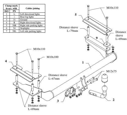
This towbar is designed to assembly in following cars: **OPEL VECTRA "B" ESTATE,** produced since 1996 till 2003, catalogue number **E27** and is prepared to tow trailers max total weight **1700 kg** and max vertical mass **75 kg**.
